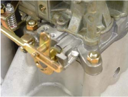
Outboard carb must be fully open.
