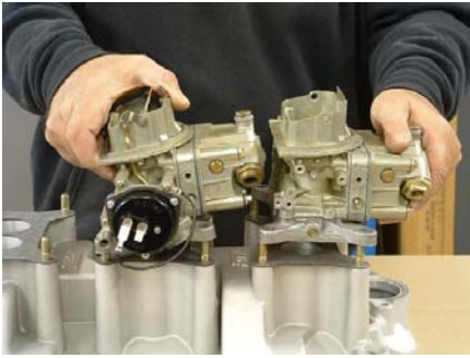
4: Install outboard carbs. You may have to tip carbs to place them on intake.
