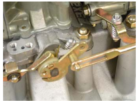
15. To adjust carb throttle, hold carbs full throttle and adjust rods so outboard carbs are fully open as shown.
