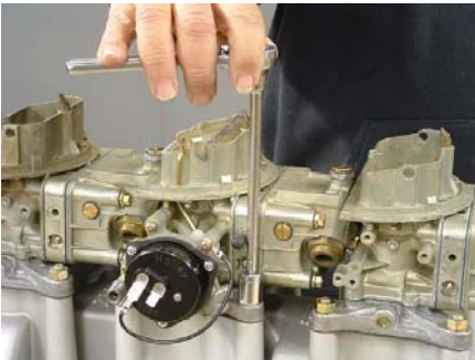
7: Once you have all carb. nuts installed, check throttle opening on each carb. then tighten nuts (caution don't over tighten).
