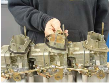
19. Place air cleaner base gaskets on all carbs.
