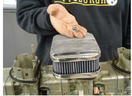
20. Place air cleaner on carbs install washer and chrome nut.
