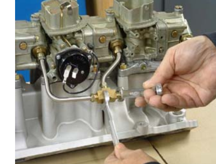
11: Once all fittings are installed finger tight, tighten with wrench.
