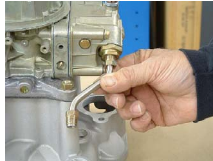
8: Install fuel lines finger tight. Do not fully tighten until all lines are installed.
