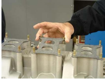
2: Install carb base gaskets.
