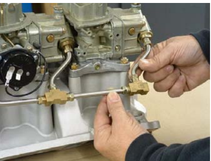
10: Continue installing fuel lines.
