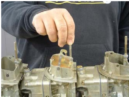
18. Place air cleaner studs in carbs and tighten. (Caution do not over tighten).
