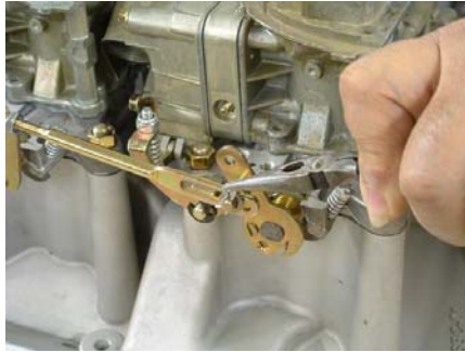
16. Place washer and wire clip in end carb throttle pins.
