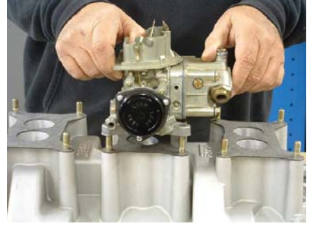
3: Install center carb (one with choke).
