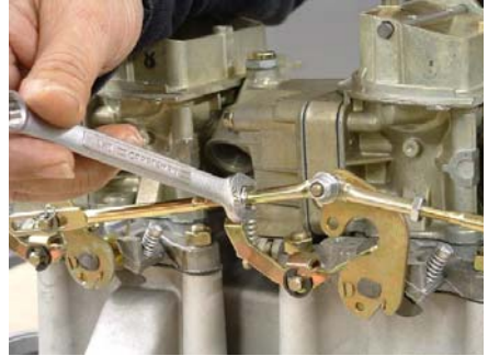
17. Tighten lock nut at this time, caution do not over tighten.
