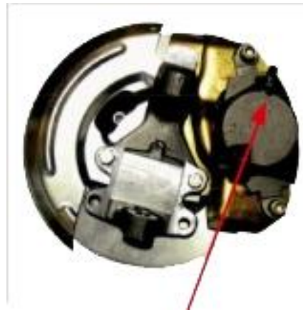
Bleeder Valves Up
