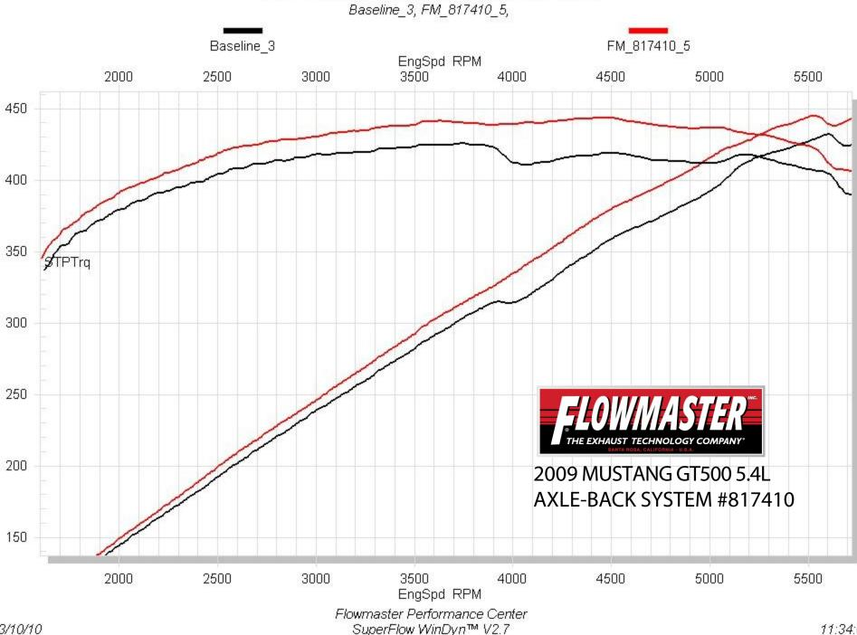
STP Corrected Wheel Power vs. RPM
