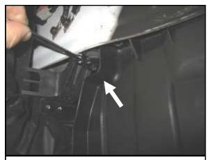
K. Remove the 6MM bolt on the frame rail holding the top of the air box resonator.
