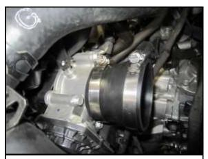
A. Install reducer coupler (B) (5-253) on the throttle body with the #40 (A) and #48 (D) hose clamp.
