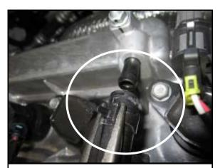
B. Release the clip on the valve cover for the PCV hose, then remove the hose from the valve cover.
