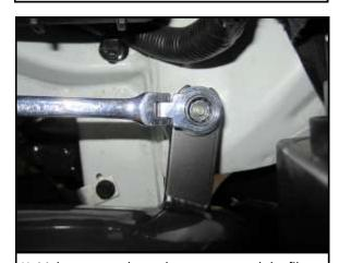
H. Make sure you have clearance around the filter and tighten the 6MM nut installed in step E.
