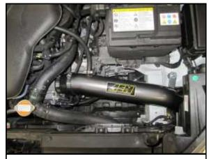
L. Check the fitment of the intake system and ensure there is clearance between the inlet pipe and its surrounding components. Once proper fitment is achieved check all the hose clamps and M6 nut on the rubber mount.
