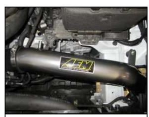
D. Install the AEM intake tube (C).
