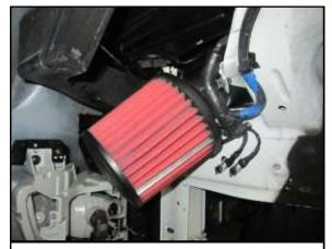
F. Install the AEM filter (E) with the #48 hose clamp.
