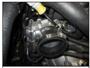
B. Tighten the #40 (A) hose clamp on the throttle body.
