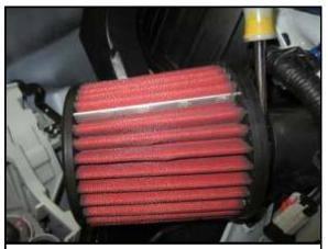
G. Rotate the AEM filter to allow for proper clearance and tighten the hose clamp on the filter.
