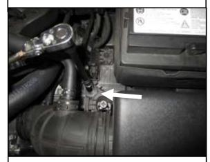
D. Loosen and remove the left 6mm bolt holding the air box.
