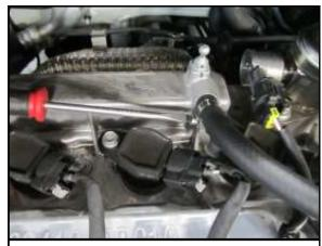
K. Install the 3/8 hose (G) and 5/8 hose clamp (F) on the PCV breather on the valve cover.
