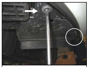
H. Remove the two lower clips on the bottom of the fender liner .
