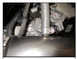
J. install the 3/8 hose (F) and 5/8 (G) hose clamp on the intake tube.
