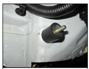
C. Install the rubber mount (J) in the OEM threaded bolt hole as shown.
