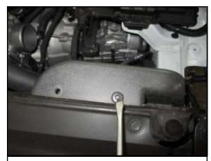
P. Push in on the center of the clips as shown and remove clips. Remove the air scoop.
