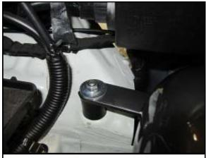
E. Install the 6MM washer (I) and nut (H) on the rubber mount.
