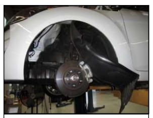
J. Move the fender liner out of the way to gain access to the resonator .
