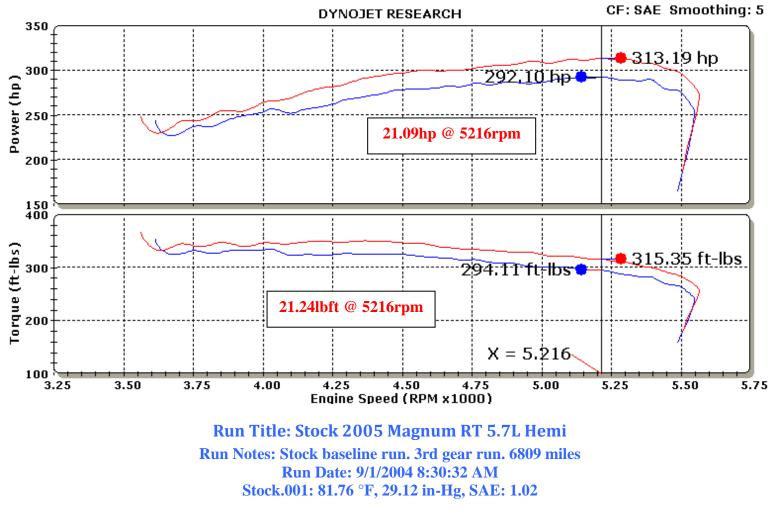
Run Title: K&N Intake Kit 2005 Magnum RT 5.7L Hemi Run Notes: K&N Intake Kit #57-1542 installed. 3rd gear run. 6809 miles. Run Date: 9/1/2004 9:52:21 AM FIPK.002: 86.64 °F, 29.07 in-Hg, SAE: 1.03
