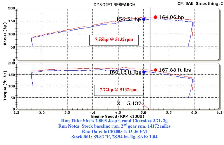
Run Title: K&N 2005 Grand Cherokee 3.7L 2g Run Notes: K&N intake kit #57-1545 installed. 2<sup>nd</sup> gear run. 14172 miles. Run Date: 6/14/2005 2:43:17 PM K&N.002: 94.86 °F, 28.93 in-Hg, SAE: 1.04
