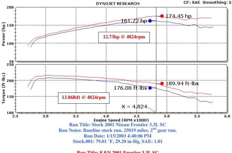
Run Title: K&N 2001 Frontier 3.3L SC Run Notes: K&N intake kit #57-6010 installed. 25019 miles. 2<sup>nd</sup> gear run. Run Date: 1/15/2003 5:37:56 PM K&N.002: 77.13 °F, 29.19 in-Hg, SAE: 1.01
