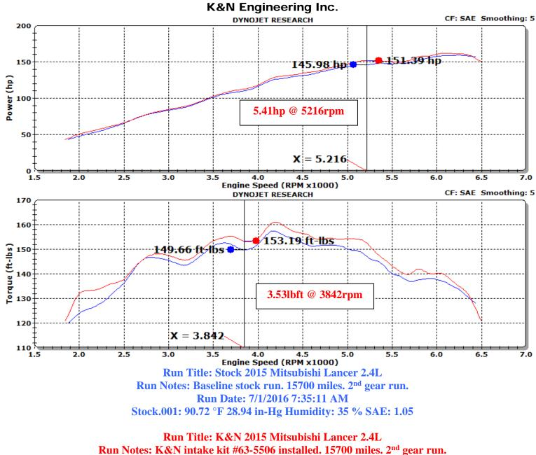
Notes: K&N intake kit #63-5506 installed. 15700 miles. 2<sup>nd</sup> gear Run Date: 7/1/2016 9:21:53 AM K&N.002: 93.63 °F 28.97 in-Hg Humidity: 33 % SAE: 1.05
