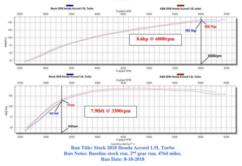
Run Title: K&N 2018 Honda Accord 1.5L Turbo Run Notes: K&N intake kit #69-1507 installed. 2<sup>nd</sup> gear run. 4764 miles. Run Date: 8-10-2018
