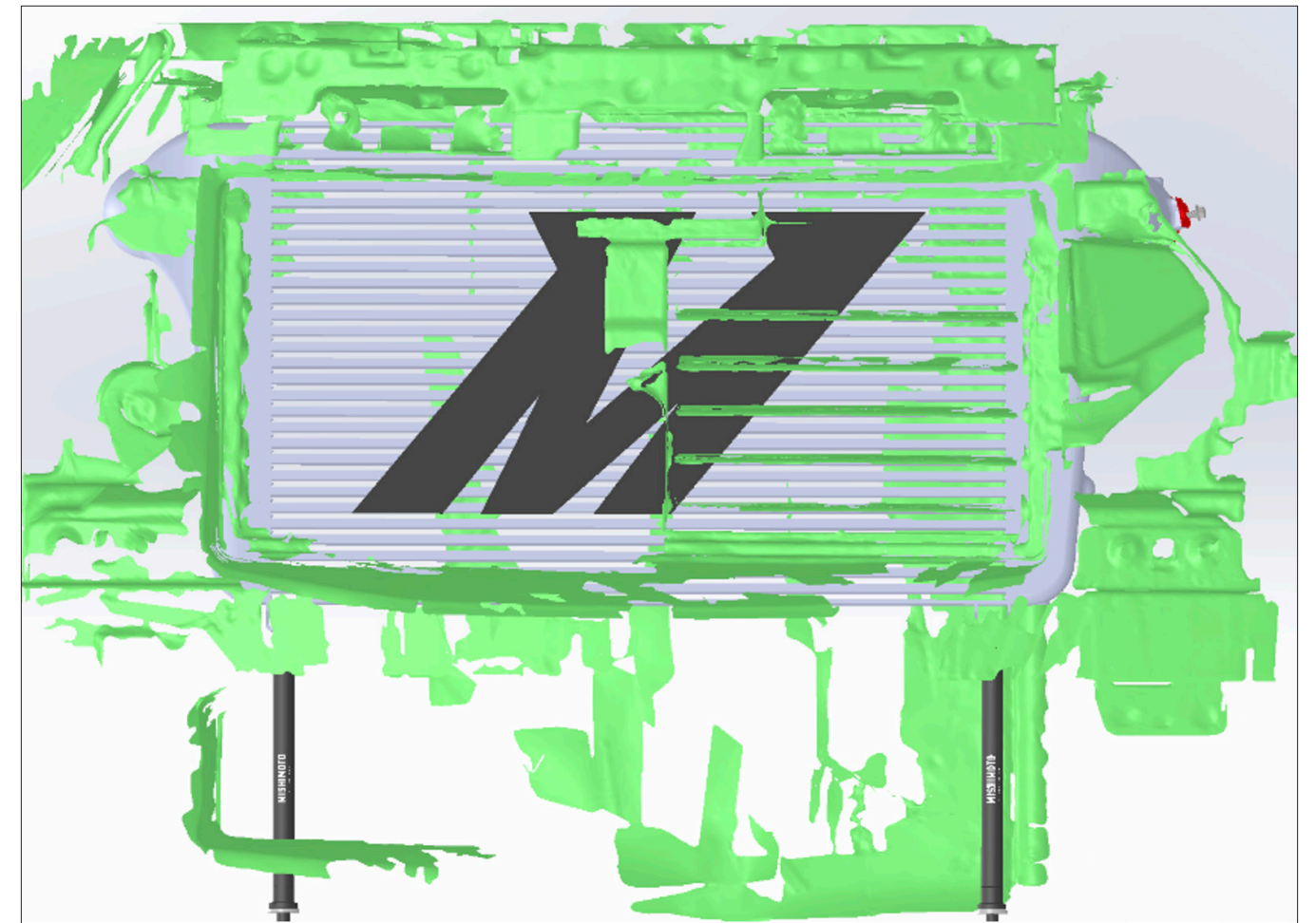
FIGURE 4: Scan Data overlaid on Mishimoto Intercooler.
