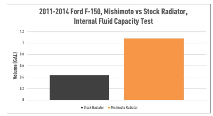
FIGURE 2: The Mishimoto radiator features an increase in coolant capacity, which promotes greater heat transfer.
