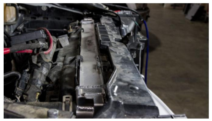
**FIGURE 1:** The F-150 radiator mounted in the truck, showing room behind the radiator.
