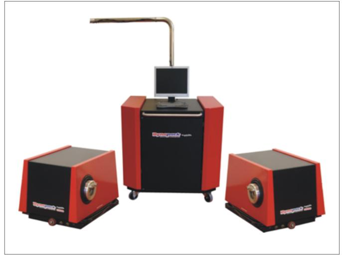
**FIGURE 5:** A Dynapack<sup>TM</sup> dynamometer was used for vehicle testing.
