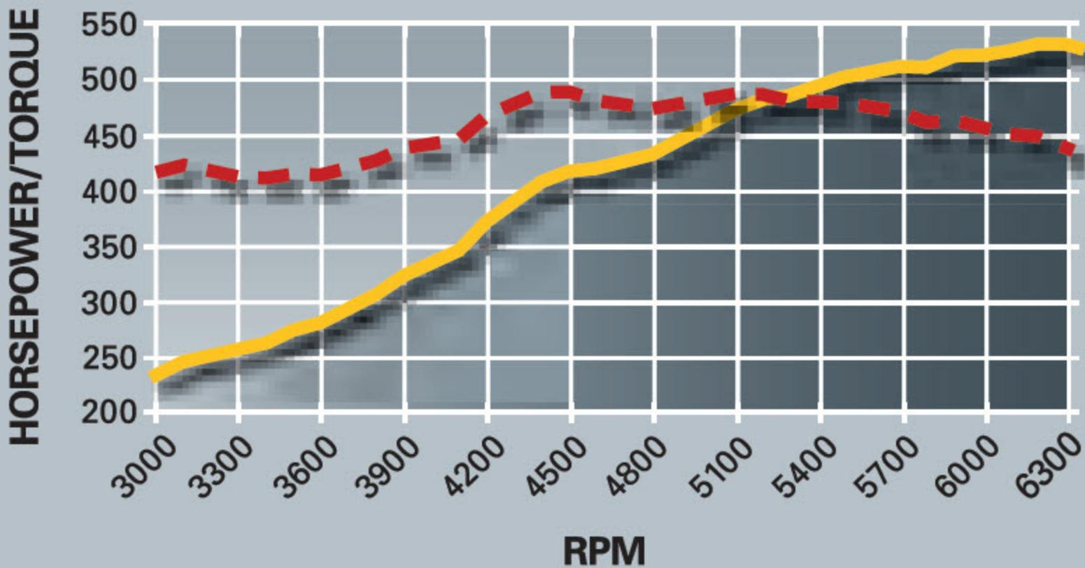
Horsepower: 525 @ 6,300 rpm
