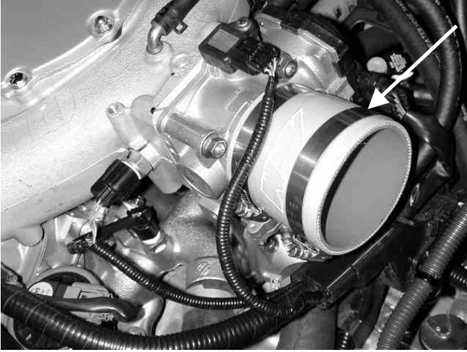
a) Install coupler onto throttle body, utilizing the supplied hose clamps.
