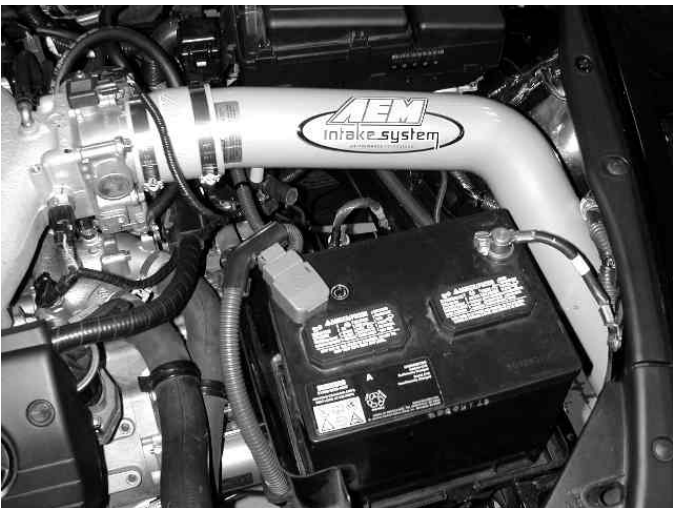
e) Place pipe into the engine bay as shown.
