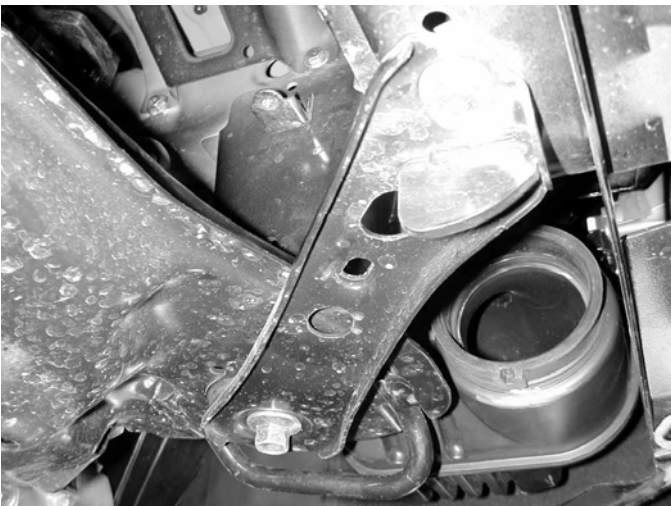
s) Pull plastic inlet pipe from air box, remove it from the vehicle.
