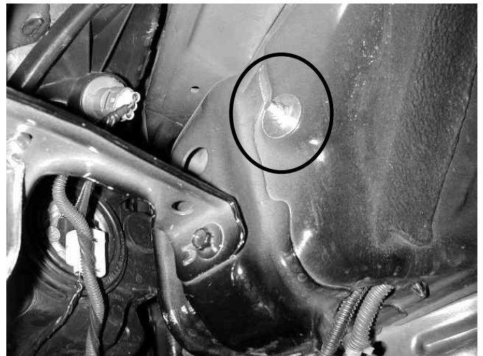
d) Secure the rubber mount stud inside the fender well with the supplied washer and lock nut.
