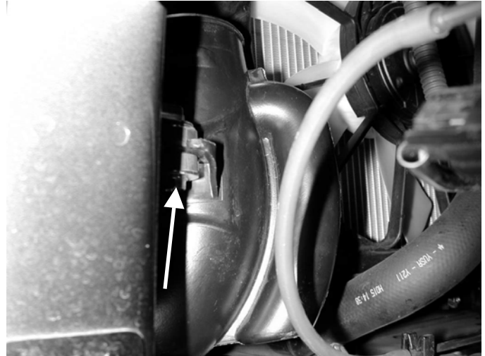
r) Cars with automatic transmissions: Loosen and remove resonator bolt.
