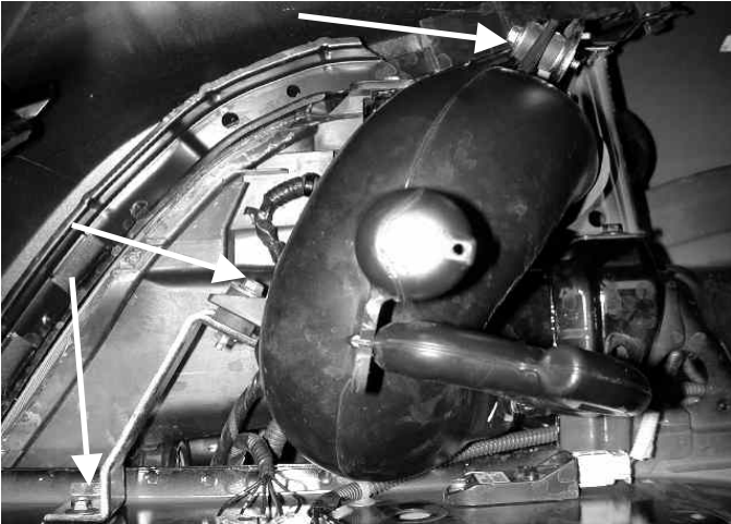
q) On manual transmission equipped cars: the stock resonator looks like the one pictured above. Remove the two mounting bolts holding it in place and the mounting bracket attached to the frame. See step 3.
