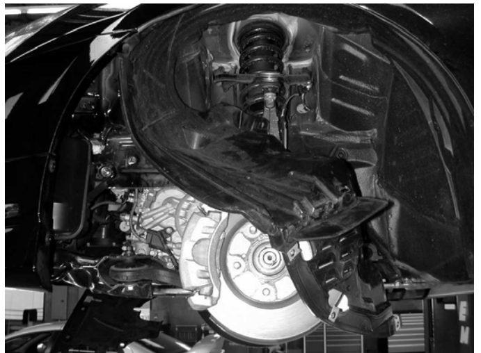
p) Place fender liner as shown.
