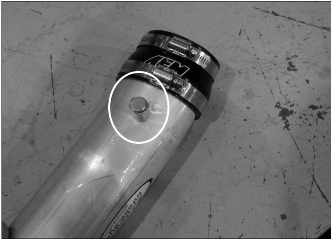
c) Insert the supplied Hex Head plug into the threaded nipple. Be sure to use the supplied O-ring.
