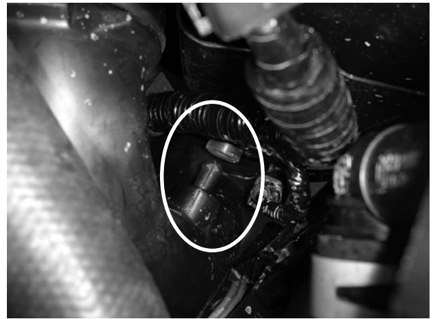
k) Pull the upper intake tube out of the grommet, located on the side of the battery box.
