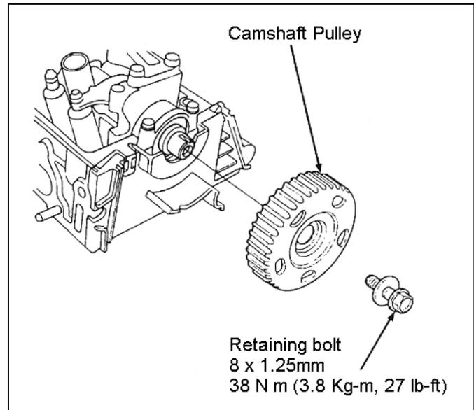
e) Remove the bolt securing the camshaft pulley. Remove the Camshaft pulley.
