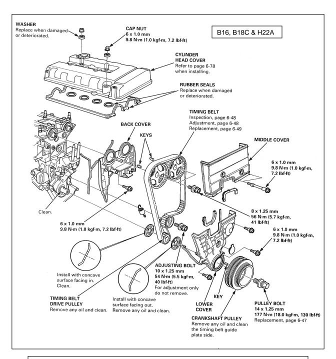
c) Remove the cap nuts, nuts and washers securing the valve cover to the cylinder head. Remove valve cover. Remove the bolts securing the middle cover. Remove the middle cover. Remove the rubber plug to expose the belt tensioner adjustment bolt.
