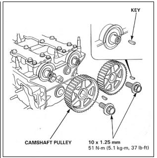
e) Remove the bolts securing the camshaft pulleys. Remove the camshaft pulleys and keyways.
