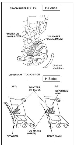
c) Align the motor to TDC. Always rotate motor in a counter-clockwise motion.
