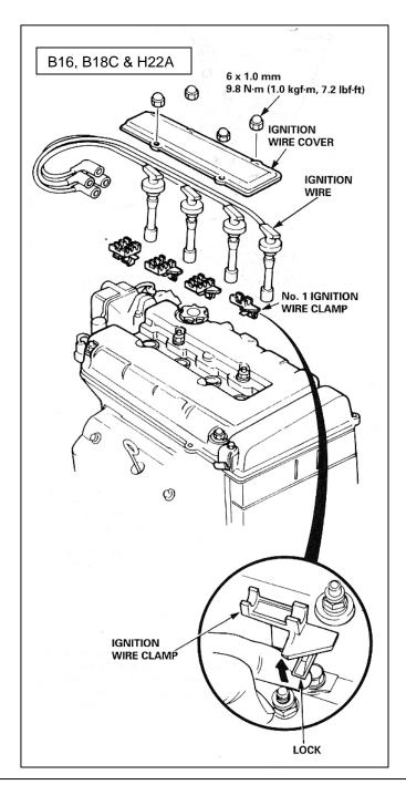
b) Remove the nuts securing the ignition wire cover. Remove the ignition wire cover. Remove the spark plug wires.
