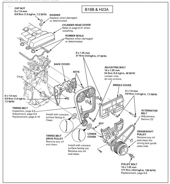
a) Remove the spark plug wires. Remove the cap nuts and washers securing the valve cover to the cylinder head. Remove valve cover. Remove the bolts securing the middle cover. Remove the middle cover. Remove the belt tensioner adjustment bolt.
