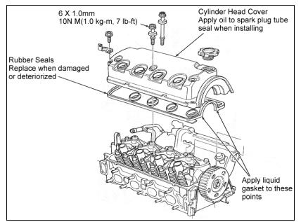
a) Remove the spark plug wires. Remove the bolts securing the valve cover to the cylinder head. Remove valve cover.
