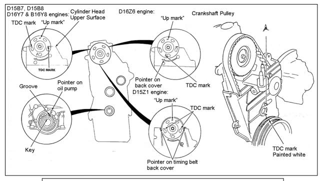
c) Align the motor to TDC. Always rotate motor in a counter-clockwise motion.
