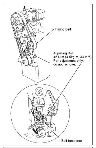
d) Loosen the belt tensioner bolt 180 degrees. Push the tensioner to release tension from the belt, and then retighten the adjusting bolt. Remove the timing belt.
