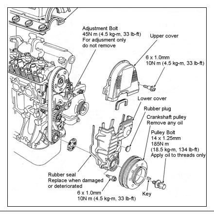
b) Remove the bolts securing the upper cover. Remove the upper cover. Remove the rubber plug to expose the belt tensioner adjustment bolt.
