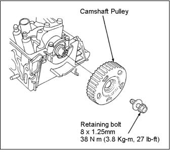
e) Remove the bolt securing the camshaft pulley. Remove the Camshaft pulley.
