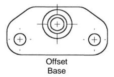
Note: Honda uses two styles of fuel pressure regulator bases. Before proceeding with your installation please compare the fuel pressure regulator on your vehicle and your new AEM adjustable fuel pressure regulator with the above diagrams.
