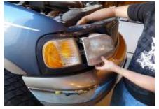
Step 3: Pull off the headlight assembly straight out from the car and unplug the headlight harness.
