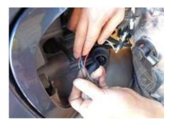
Step 7: Splice in the halos into the corner light. Halo wires are two red one power and the other wire ground. Splice one red wire (+) positive into the brown wire on the corner light. Other red wire (-) negative will be spliced into the black wire on the corner light.
