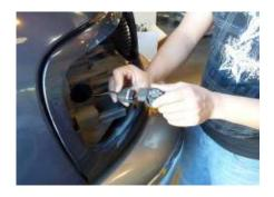
Step 6: Remove corner bulb out from the harness.
