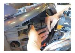
Step 9: Plug in the headlight harness into the new Anzo headlight assembly.
