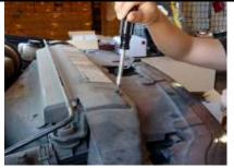
Step 1: Remove the eight plastic screws holding in the plastic cover shroud.
