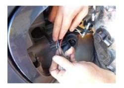
Step 8: Splice the led wires into the corner light. Blue wire (+) will be positive splice into the brown wire on the corner light. Black wire (-) negative will be spliced in to the black wire on the corner light.
