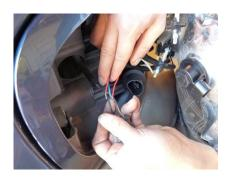
Step 7: Splice in the halos into the corner light. Halo wires are two red one power and the other wire ground. Splice one red wire (+) positive into the brown wire on the corner light. Other red wire (-) negative will be spliced into the black wire ont he corner light.
