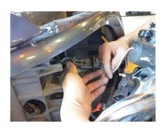
Step 9: Plug in the headlight harness into the new Anzo headlight assembly.
