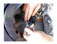
Step 8: Splice the led wires into the corner light. Blue wire (+) will be positive splice into the brown wire on the corner light. Black wire (-) negative will be spliced in to the black wire on the corner light.
