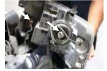
Connect the headlight, signal, and side marker harness into its power source sockets
