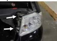
Remove the grille shroud and expos the two 10mm bolts on the side of the OEM headlight
