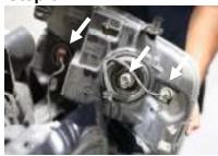
Remove the OEM headlight by removing the headlight, signal and side marker bulb housing
