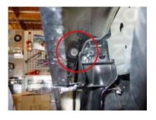
Step 6: Remove the 10mm bolt located inside the fender behind the headlight housing.
