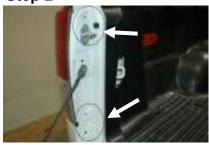
Remove the two phillips screws located directly behind the tail light housing
