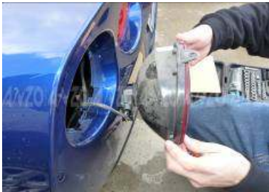
Step 2: Remove the tail light from the bumper.
