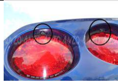
Step 1: Unscrew the two torque screws located at the top of the tail light.
