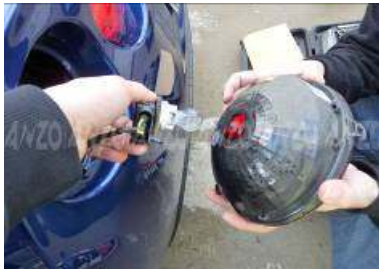
Step 3: Twist off the light bulb socket.
