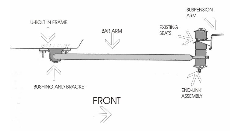
DUE TO A CHANGE IN THE U-BOLT, THE BASE PLATE HAS BEEN OMITTED.
