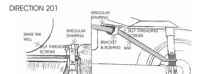
Step #1. With the car resting naturally on its springs, pass the bar over the exhaust from one side with the wheel removed. Position the bar so it passes 1/2 inch forward of the spare tire well with the arms forward over the axle.
