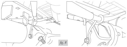
Wire bracket on emergency brake cable (F-250)
