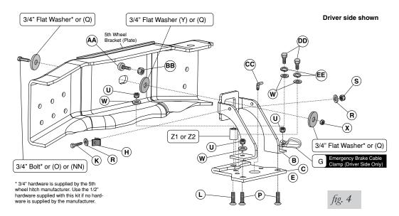
1. Set the upper brace (B) into the driver and passenger side frame (fig. 4).
