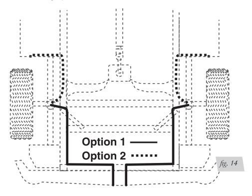
7. Cut off the air line, leaving approximately 12" of extra air line. A clean square cut will ensure against leaks. Insert the air line into the air fitting. This is a push-to-connect fitting. Simply push the air line into the 90° swivel fitting until it bottoms out (9/16" of air line should be in the fitting).
