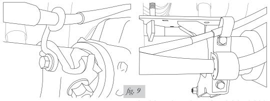
Wire bracket on emergency brake cable (F-350)
