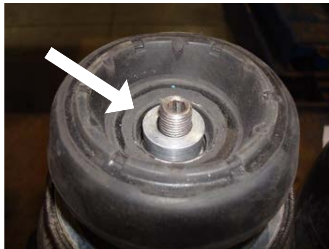
Rubber removed from VR6 mount
