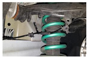
10. Remove the brake line bracket from the body (dual motor vehicles only).
