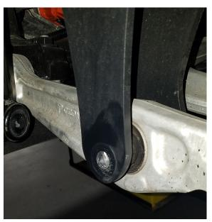
12. Loosen and remove the upper ball joint retaining bolt. Separate the ball joint from the knuckle.
