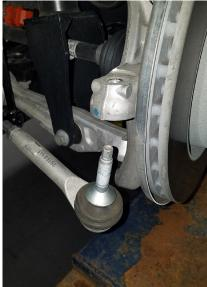
9. Remove the ABS sensor wire from the upper control arm by releasing the clips from the control arm mounting points.
