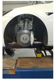
7. Remove the stabilizer bar end link from the strut tab.
