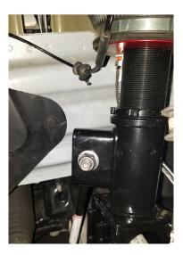
8. Reinstall the ABS sensor wire clips on the upper control arm.
