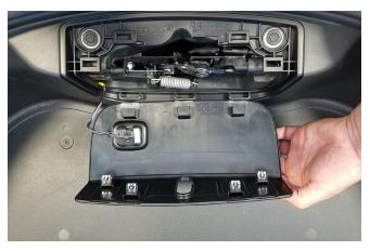
4. Remove the attaching bolts for the underhood luggage compartment. Then remove the underhood luggage compartment from the vehicle.
