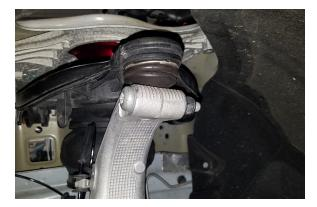
5. Raise the lower control arm and reinstall the lower shock mount bolt and nut hand-tight. Do not torque the bolt at this time.
