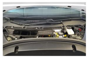
2. Remove the cabin intake duct by pulling up to release the clips.
