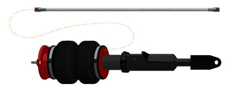
2. Using the (3) previously removed upper shock mount nuts, install the Air Lift Performance shock on the upper control arm mount and torque the nuts to 23Nm (17 lb.-ft.).
