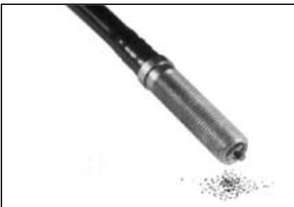
Leak test the inflation valve for leaks at the air line connection or dirt or debris in the valve core. See page 7 for repair.
