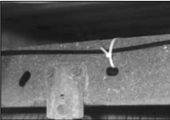
Inspect air lines to be sure it is not pinched. Tie straps may be too tight. Replace strap.
