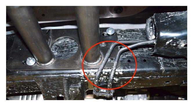
7.) On the driver side, the KDSS brackets removed in step 4 will be reinstalled on top of the rear slider plate.
