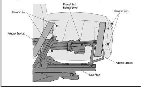
Note: In order to tumble the seat forward to access the rear of the vehicle, reach under the seat and manually push down on the Seat Release Lever.
