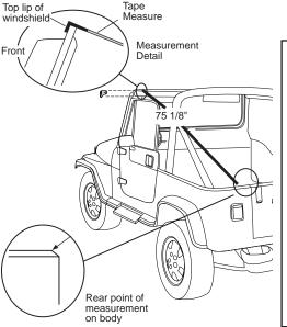
Wrangler/YJ Windshield Adjustment: If necessary, loosen the #40 TORX bolts in the windshield clamps to loosen the windshield in order to slip the bracket under the horizontal tube.
