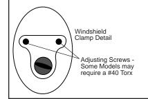
Under most circumstances, the wind-shield of the Wrangler will not require any adjustment. If your Wrangler windshield should require adjustment, this adjustment should be performed only by an authorized automotive mechanic using a special "Tamper-Proof" Torx head tool.
