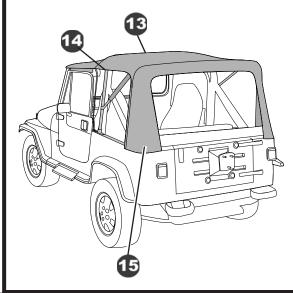
Snap the tab just behind the door opening on each side of the vehicle to the studs on the center bow.
