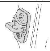
Special Note: The Rotary Latch Paddle Handlevill only latch on the automobile manufacturer's original equipment steel latch pin located on the vehicleDo Not adjust or remove this part.
