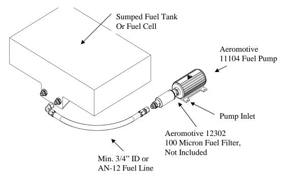
Note: If you would like a fuel shut off valve installed between the fuel tank outlet and the fuel pump. Use Aeromotive part # 12332 shutoff valve fuel filter in place of the 12302 fuel filter.
