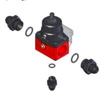
20. Install one AN-08 o-ring on the port (cut-off) side of each of the four P/N 15607 ORB-08/AN-08 port fittings.
