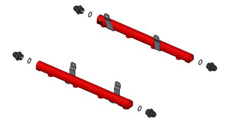
22. Inspect the o-rings on the OEM quick disconnect fitting for both supply and return line and replace if necessary. Coat o-rings and the adapter fitting with a light oil and install the P/N 15101 AN-06 / Ford quick disconnect adapter fitting on the OEM return (bypass) fuel line.
