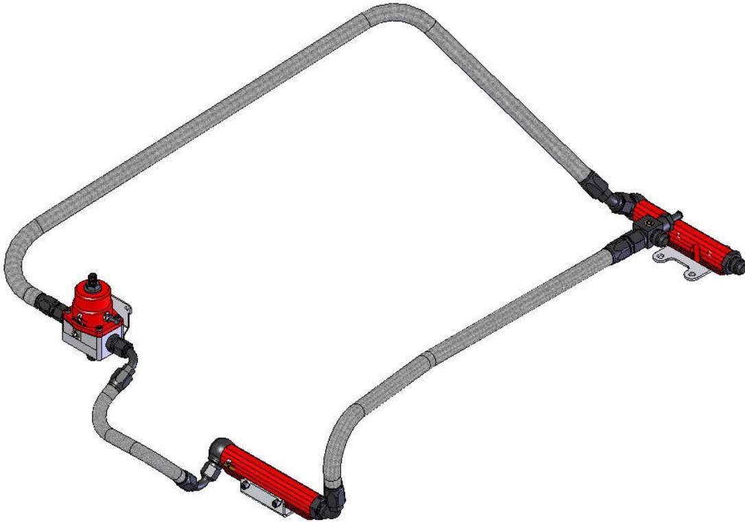
39. Connect one of the AN-08 45-degree hose ends to the front of the driver (left) side fuel rail and an AN-08 90-degree hose end to the 90-degree AN-08 male flare on the fuel supply tee adapter. Plan a route for the line between the fuel rail and the supply tee adapter, measure the length of fuel line needed and cut. See section titled Hose and Fitting Assembly for fuel line assembly instructions. Once the hoses are assembled, **ensure there is no debris in the hose** and install it.
