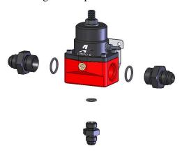
29. Install one ORB-08 o-ring on each of the two ORB-08/AN-08 port fittings.
