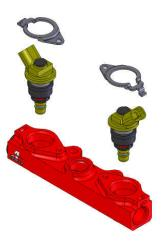
21. Reinstall the injector retaining clips and tighten screws.
