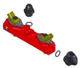
32. Thread the o-ring side of two of the ORB-08/AN-08 port fittings into the top center port, and in the front port, of the driver side fuel rail.
