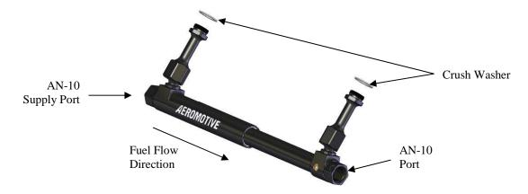
5. With the fuel log in place pivot the log to the position that provides the most clearance and tighten the pivot nuts to 20 in-lbs.
