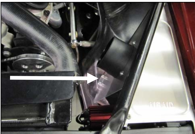
13. Secure the Air Dam tab to the inner fender using the two Self drilling screws (#8).
