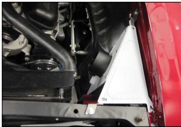
8. Position the airbox assembly into the inner fender area. Check for clearance and adjust the panels and brackets for fit, and tighten all hardware, final tight.
