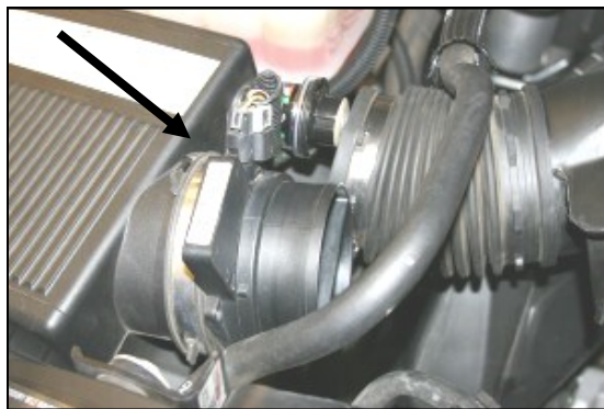
2. Remove the factory tube from the Mass Air Sensor, and slide it out of the way. Next loosen the hose clamp on the Mass Air Sensor.
