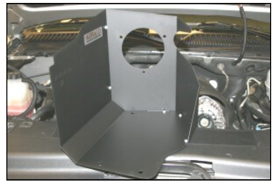
6. Assemble the two Cool Air Dam panels (#2) and (#3) using the five supplied screws (#9), washers (#10), and nuts (#11), as shown.
