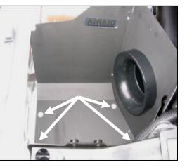
**8.** Position the Airaid Cool Air Dam in place of the factory air box. Secure it to the factory mounting pad using four M6-1x25 bolts (#11) and <sup>1</sup>/<sub>4</sub>" flat washers (#10). (<u>Caution</u>: over tightening may distort the cool air dam!
