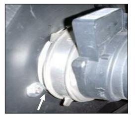
9. Slide the factory MAF meter onto the filter adapter. Tighten the hose clamp. (*Note: The factory clamp / rubber bushing must be in place on the inlet to the MAF meter.*) Reconnect the factory intake tube, MAF meter wiring harness, and tighten the clamps.
