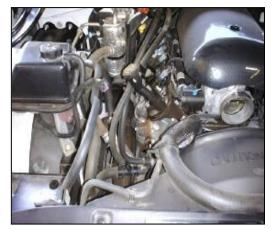
**3.** Remove the factory air filter lid, intake tube, and base from the vehicle as an assembly. (Hint: pull straight up on the air filter base to remove, there are no bolts, just grommets).
