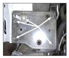
4. Using a 10mm socket, remove the five
