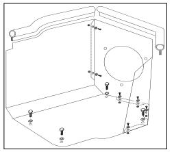
**5.** Assemble the Airaid Cool Air Dam pan-
