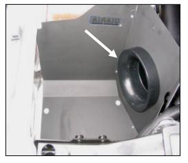
7. Install the filter adapter (#4) using three  $\frac{1}{4}$ -20 x  $\frac{1}{2}$ " button head bolts (#9) and  $\frac{1}{4}$ " flat washers (#10).
