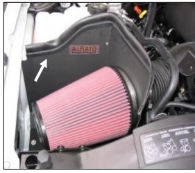
**10.** Mount the Airaid Premium Filter (#1) onto the filter adapter and tighten the hose clamp. Press the weather strip (#5) along the top edges of the Airaid cool air dam; assure that it is fully seated along the edges. (Hint: *Begin at a corner and work toward the ends*).
