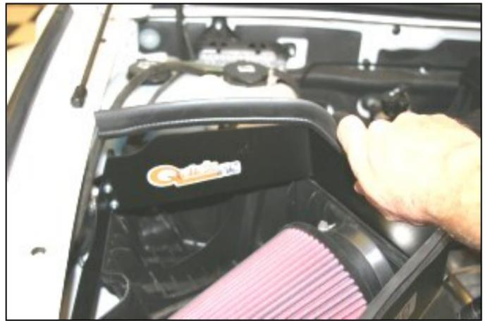
8. Starting at one end of the Quick Fit Panel, install the weather strip (#4) as shown.
