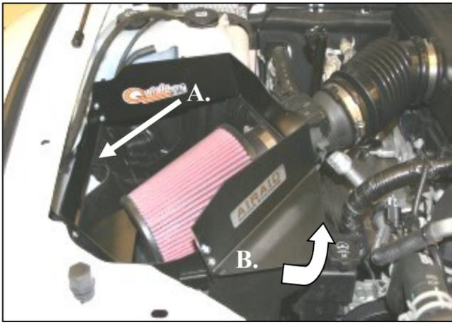
7. **A.)** There are two tabs on the Quick Fit Panel, insert the one closest to the headlight first into the slot on the factory airbox.
