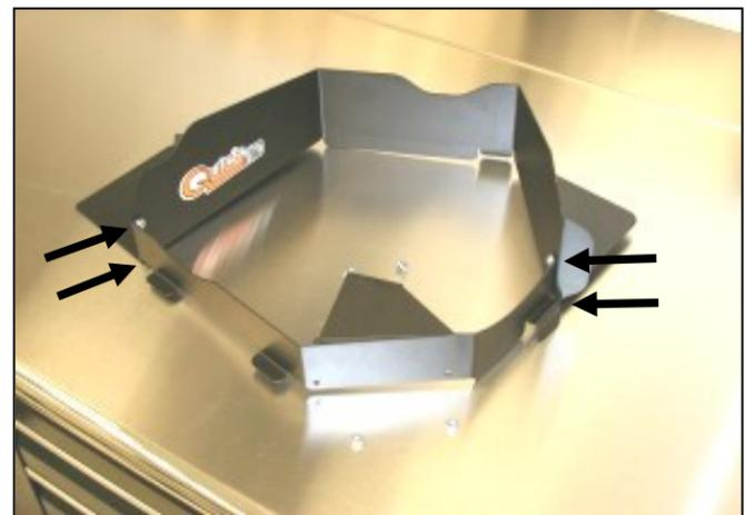
4. Assemble the Airaid Quick Fit Panels (#2, #3) using four 6-32x 5/16" screws (#5), #6 flat washers (#6), and 6-32 keps nuts (#7).
