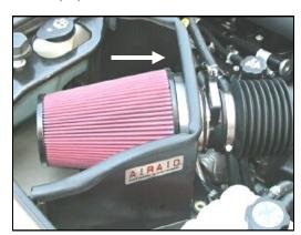
**8**. Install the Airaid Premium Filter (#1) onto the filter adapter, and tighten the hose clamp. Install the provided weather strip (#5) onto the top edge of the panel. (Hint: Start at one end, and work to the other.)
