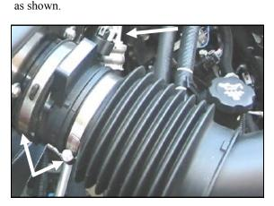
7. Slide the MAF sensor onto the filter adapter and tighten the clamp. Slide the factory intake tube onto the other side of the MAF sensor, and tighten the clamp. Reconnect the MAF sensor wiring harness.
