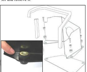
**4.** Assemble the Airaid Cool Air Dam panels (#2, #3) using the factory rubber grommets and inserts
