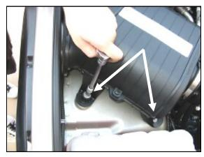
**2.** Using a 10mm socket, remove the three bolts that secure the factory airbox to the inner fender (save for reuse).
