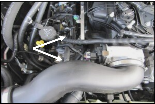
12.) Install the 3/8" Breather Hose (#7) onto the Barbed Fitting and factory hard line.
