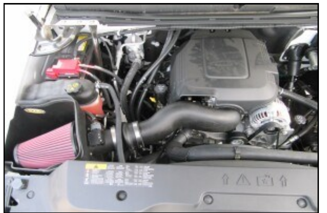
14. Reinstall the engine cover. Double check your work! Make sure there is no foreign material in the intake path. Make sure all clamps, hoses, bolts, and screws are tight. Double check the hood clearance. Reconnect the negative battery cable
