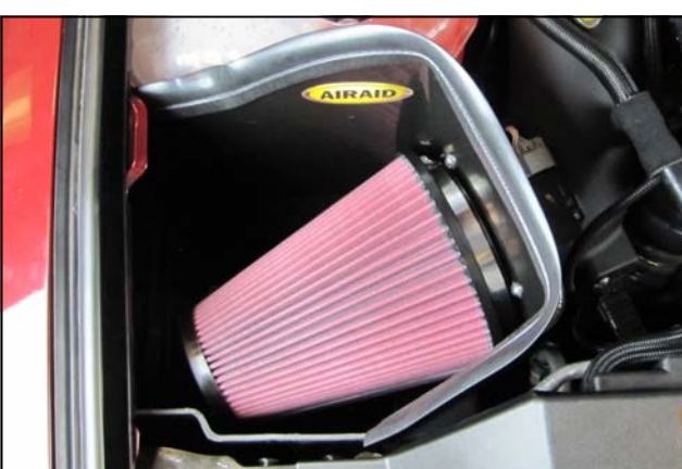
17. Install the Airaid Premium Filter onto the Intake Tube inside of the Cold Air Box. Install the Weather Strip onto the top edge of the Cold Air Box with the contour rolling away from the filter.
