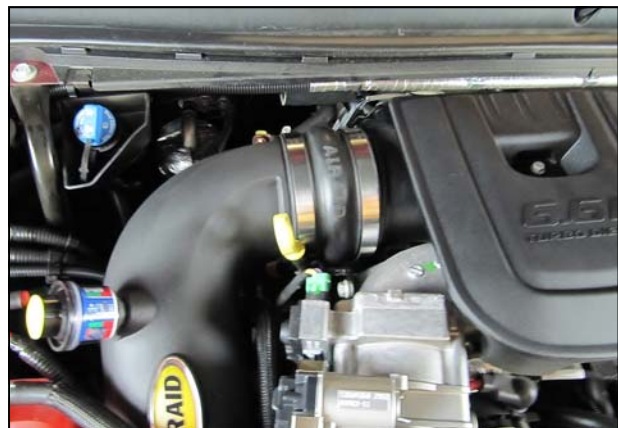
15. Tighten the two Hump Hose Clamps. On the turbo inlet.
