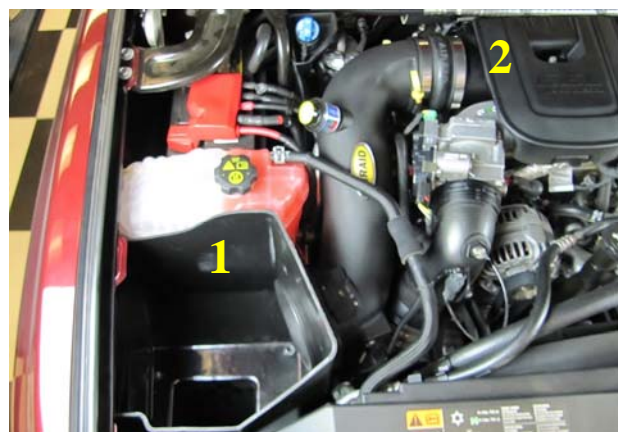
12. Slide the Intake Tube down and into the Cold Air Box, then into the Hump Hose on the turbo inlet.
