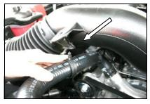
1. <u>Disconnect the negative battery cable!</u> Lift up on the front of the and beauty cover and remove it from the vehicle. Push down on the radiator hose, and separate the tube from the plastic clamp.
