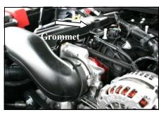
**9.** Re-install the intake tube using caution to center the intake tube hole over the previously installed grommet. Some adjustment may be required to seat the grommet correctly back into the intake tube. Tighten the hose clamps on the tube. Re-connect the breather tube. Re-install the plastic holder from step #1. Re-install the beauty cover.
