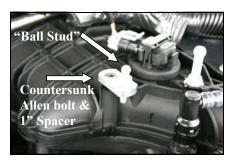
6. Remove the "ball stud" from the top of the intake manifold, insert the countersunk Allen bolt (#6) thru the countersunk hole in the provided 1" spacer plate (#5). Thread the countersunk bolt into the hole where you removed the "ball stud", face the spacer towards the front of the vehicle, and tighten the countersunk Allen bolt. Next thread the "ball stud" into the forward hole in the 1" spacer and tighten.
