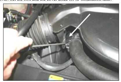
**3.** With a screwdriver, pry the factory tube away from the plastic tab on the radiator hose clamp, and remove the tube.
