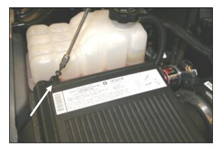
**8.** If you purchased the 200-719 Jr. Kit, remove 4 screws in the factory airbox with a #25 Torx bit, and remove the factory air filter.
