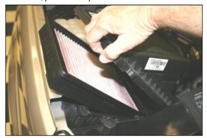
**9.** Install the Airaid Premium filter into the factory airbox, and re-install the 4 screws.
